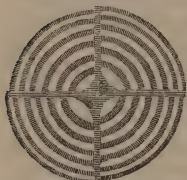
Rings and Cross of Calcareous Spar produced by circularly polarized light.
